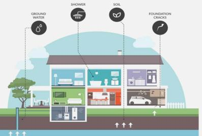
Radon may enter buildings through cracks in the floor, gaps in construction, windows, drains, or spaces around cables and pipes.
