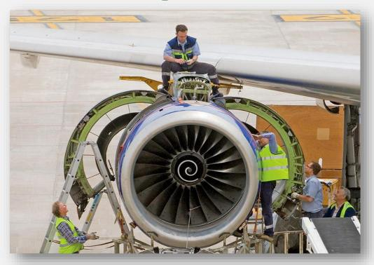
Always use fall protection equipment when working at heights and use proper maintenance stands which are more stable than ladders.
